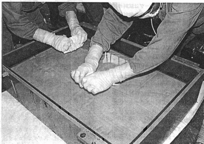
Fig. 4 Polishing work of glass slab
